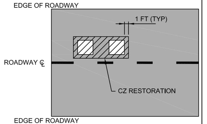
\* CONTINUOUS ZONE (CZ) RESTORATION REQUIRED WHEN ℄ OF TRENCH OPENNINGS ARE <10 FEET APART OR IF OUTER EDGE OF TRENCH OPENNINGS ARE <6 FEET APART.
