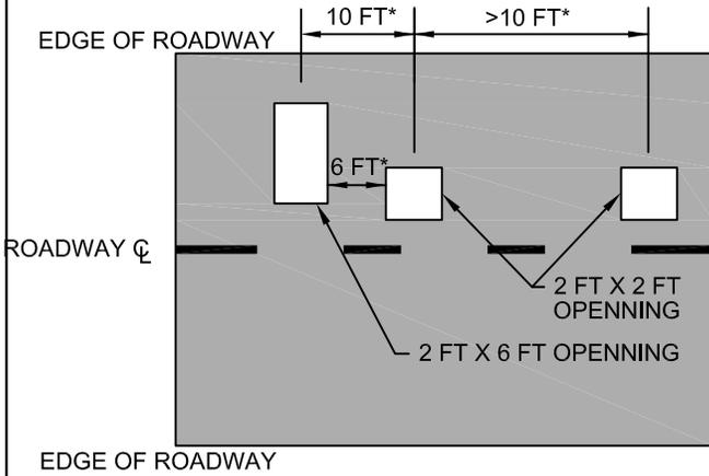
CONTINUOUS ZONE (CZ) RESTORATION: SAWCUT AND COLD PLANE MINIMUM 2 INCH DEPTH, REMOVE TEMPORARY PAVEMENT TO GRAVEL BASE UNLESS OTHERWISE APPROVED BY DPW, PLACE PERMANENT PAVEMENT.
