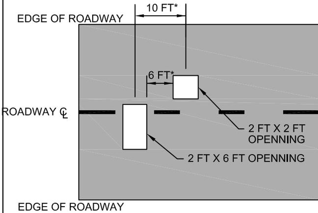
CONTINUOUS ZONE (CZ) RESTORATION: SAWCUT AND COLD PLANE MINIMUM 2 INCH DEPTH, REMOVE TEMPORARY PAVEMENT TO GRAVEL BASE, PLACE PERMANENT PAVEMENT.
